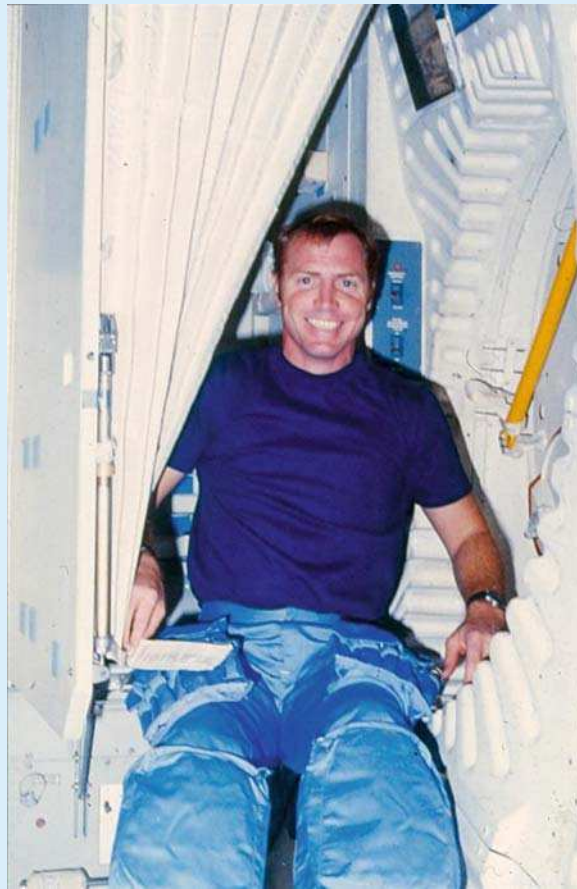
FIGURE 7.2 Astronaut David Walker demonstrating the Shuttle potty. It works by using air instead of water to move materials (NASA photograph).
